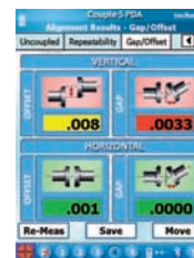
Step 4 - Gap/Offset-Results Screen Shows misalignment results instantaneously against the user-selected tolerance.
